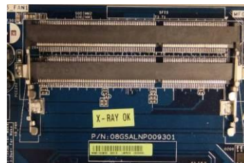
204-pin DDR3 SO-DIMM sockets
